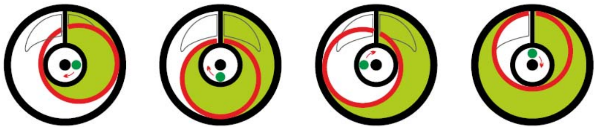
Figure 1 — Operation of Eurosens flow measuring chamber
