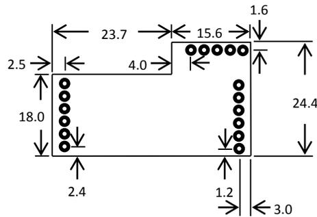
All dimensions in mm. All pinheader pitch is 2.54mm.
